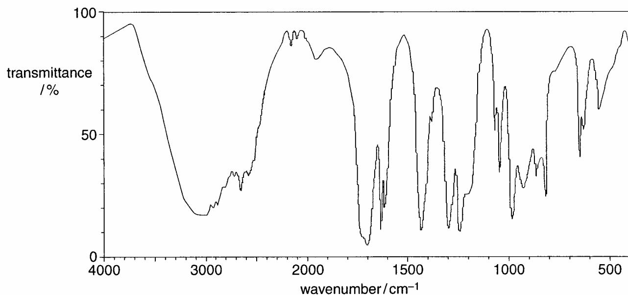
By referring to your *Data Sheet*, decide whether acrolein,  $\text{CH}_2=\text{CHCHO}$ , or acrylic acid,  $\text{CH}_2=\text{CHCOOH}$ , was formed.
